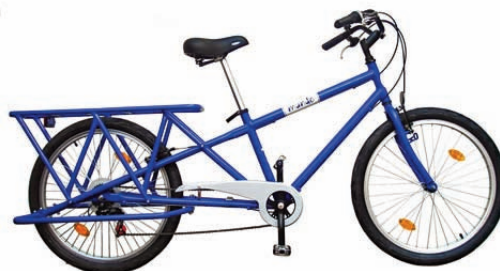
Thanks to our own John Chiarella who saw this on the web, the Mundo cargo bike, made by Yuba, a German bike company, is used for non-racing, utility purposes. A larger frame and larger wheelbase allows more rear cargo space. Website: www.yubaride.com
